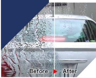
An innovative application done with special chemical compounds which goes inside the pores of the glass, reacts chemically with it and make the surface HYDROPHOBIC. It simply means that the water doesn't stick on the glass surface the keeps it almost dry and dust free.
